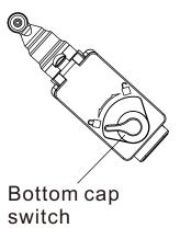
When you open the bottom cover, rotate the button to theunlocking position, then pull up the bottom cover.
